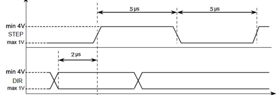
Img 8. STEP and DIR input signals
