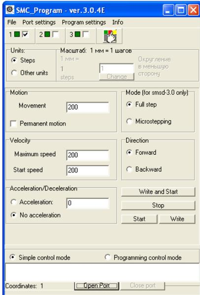
Img. 10. SMC\_Program – control via simple panel
