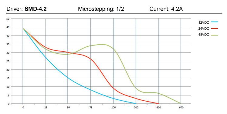
x axis - rotation speed, rpm;
