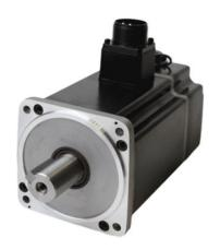
The output power of 3000 W fits into a servo motor EM3A-30 with a flange size 130 mm. This motor has low rotor inertia and high speed, suitable for highly dynamic systems. Movement accuracy is ensured by modern optical or magnetic encoders with a resolution of up to 23-bit. Products can be provided with a 24VDC holding brake option.
