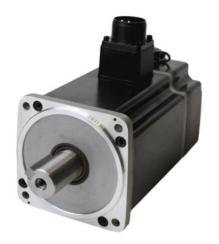
The output power of 4000 W fits into a servo motor EM3A-40 with a flange size 130 mm. This motor has low rotor inertia and high speed, suitable for highly dynamic systems. Movement accuracy is ensured by modern optical or magnetic encoders with a resolution of up to 23-bit. Products can be provided with a 24VDC holding brake option.
