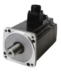
The output power of 5000 W fits into a servo motor EM3A-50 with a flange size 130 mm. This motor has low rotor inertia and high speed, suitable for highly dynamic systems. Movement accuracy is ensured by modern optical or magnetic encoders with a resolution of up to 23-bit. Products can be provided with a 24VDC holding brake option.
