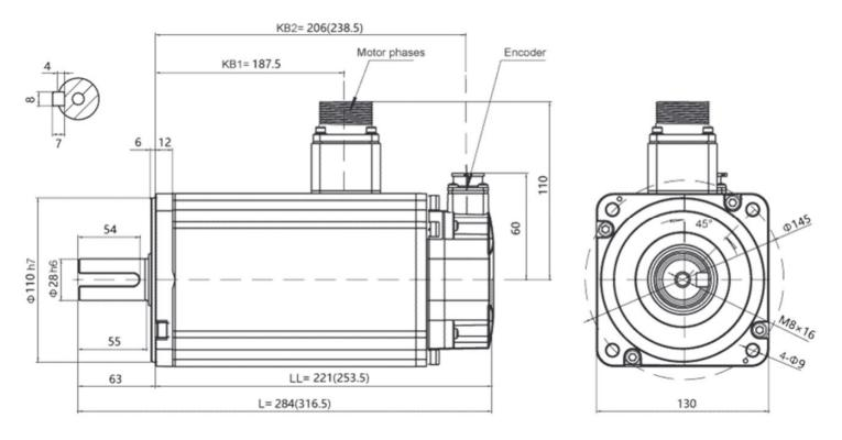
Note: The values in parentheses represent the values of motors with brakes
