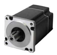
EM3A-A5 series are high speed and low inertia synchronous AC servo motors by Estun manufacturer. These small-sized servo motors with a power of 50 W are used in small automatic machines, instruments and machine tools. Motors are available with optical 23-bit or magnetic 17-bit absolute encoder. The motors are suitable for applications with a maximum speed of 6000 rpm. Products can be provided with a 24VDC holding brake option.
