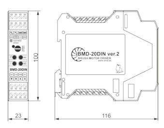
BMD-20DIN ver.2 is a DC brush motor speed controller. The controller provides different methods of motor speed regulation, using potentiometers, analog or PWM signal. Acceleration and deceleration time are also adjustable. This motor speed controller provides current limitation function to prevent motor overloading.
