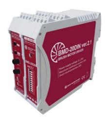
BMD-20DIN ver.2.1 is a device designed to control rotation torque, speed, direction and acceleration of a DC brush motor. The controller provides a motor overload protection function with adjustment of the maximum permissible current value. A brake control function is provided. A function of switching during operation to a second preset speed by an external discrete signal is implemented.
