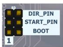
Fig. 5. START_PIN and DIR_PIN jumpers.
