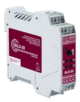
BLDC driver BLD-20DIN is a device designed to control 3-phase DC motors with Hall sensors. BLD-20DIN controls motor speed, acceleration and deceleration, direction. The controller has current limiting function to protect a motor.
