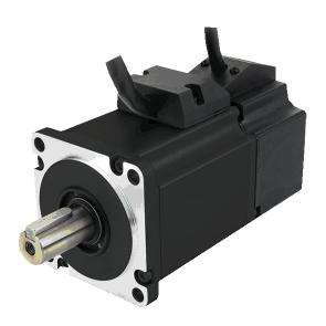
With rated power of 200 W, the high-performance BLDC motor APBA60M048030-E not only matches the power of AC servo motors with 60 mm flange but are also mechanically compatible. The DC motors are rated IP65 and comes standard with integrated encoder. The incremental encoder resolution is 2,500 CPR (10,000 PPR).
