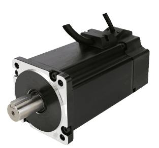
With their rated power of 1,000 W, the high-performance BLDC motor APBA80L048030-E not only matches the power of AC servo motors with 80 mm flange but are also mechanically compatible. It is rated IP65 and comes standard with an integrated encoder. The incremental encoder resolution is 2,500 CPR (10,000 PPR).
