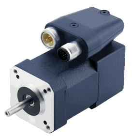
NEMA 17 BLDC motor in size NEMA 17 (42 mm) with protection class IP65 (except shaft output). With M16 and M12 connectors for power and rotary encoder.
