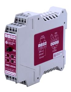
BMD-20DIN is a driver designed to control speed, direction, acceleration and deceleration of DC brush motors.
