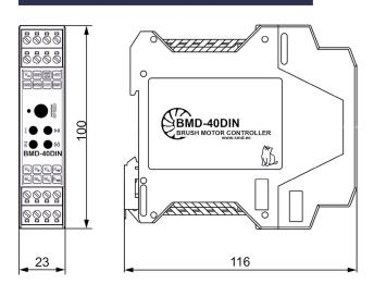
BMD-40DIN is a driver designed to control speed, direction, acceleration and deceleration of DC brush motors.
