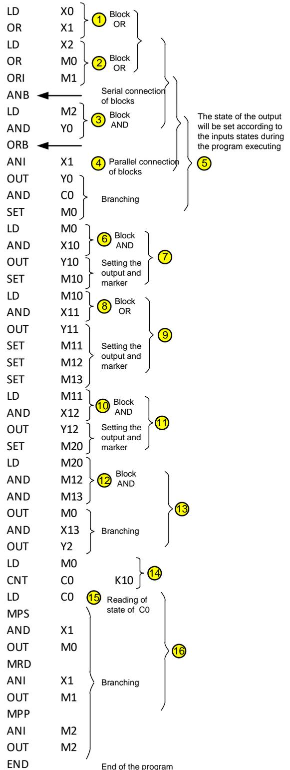
Fig. 21 – Converting of LD into IL
