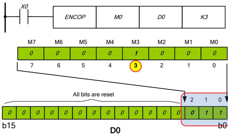
If  $2n = 23 = 8$  then output relay addresses are M0...M7. As the 3d output is turned on (i.e. M3 = 1), the value 3 is written to the data register D0.
