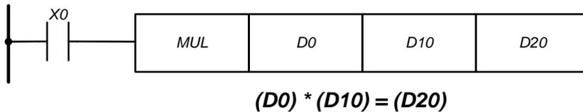
If X0 is turned on, the values in data registers D0 and D10 are multiplied together. The result is saved in the data register D20.
