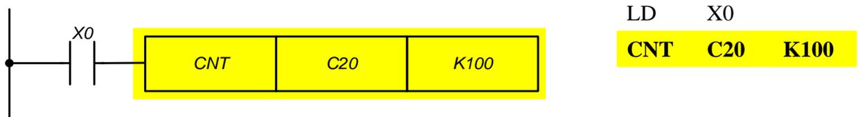
When X0 changes from "0" to "1" the value of the register C20 increases by 1. It repeats until the value of register C20 reaches K100 (100 pulses). After that the count stops, the contact C20 turns on. To reset the value of the register C20 use the instruction RST C20.
