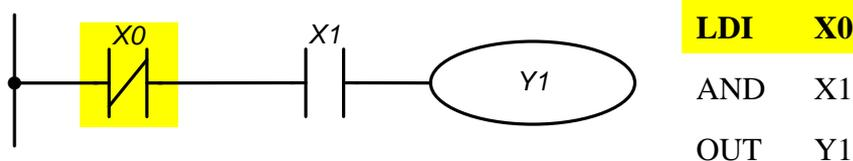
The instruction LDI X0 "normally closed contact X0" starts the sequential logic connection. If at the inputs X0 and X1 there is simultaneously a signal "1", then the output Y1 will be set to the state "1".
