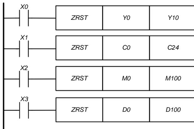
When the entry conditions are satisfied, the bit operands Y0 ... Y10, M0 ... M100 are turned off (turns to the state "0"). The numeric operands C0 ... C24, D0 ... D100 are turned to actual value "0". The corresponding coils and contacts are switched off.
