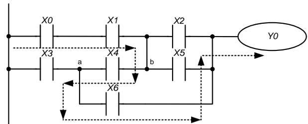
Fig. 15 – relay-contact circuit of the controller
