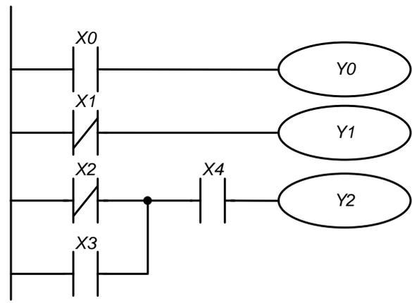
Fig. 10 – ladder diagram in the controller
