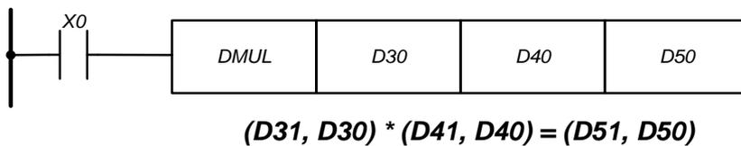
If X0 is turned on, the values in registers (D31, D30) and (D41, D40) are multiplied together. The result is saved in the data registers (D51, D50).
