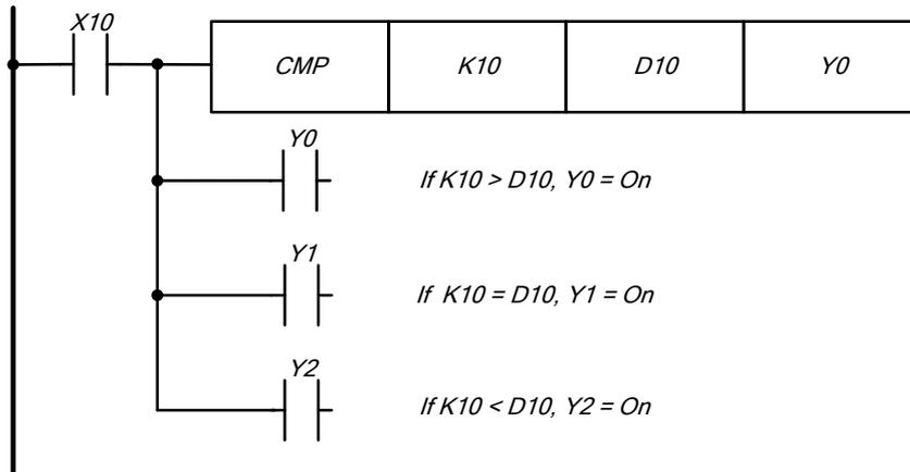
Y0: is turned on if  $K10 > \text{data register } D10$ , Y1 and Y2 are turned off.
