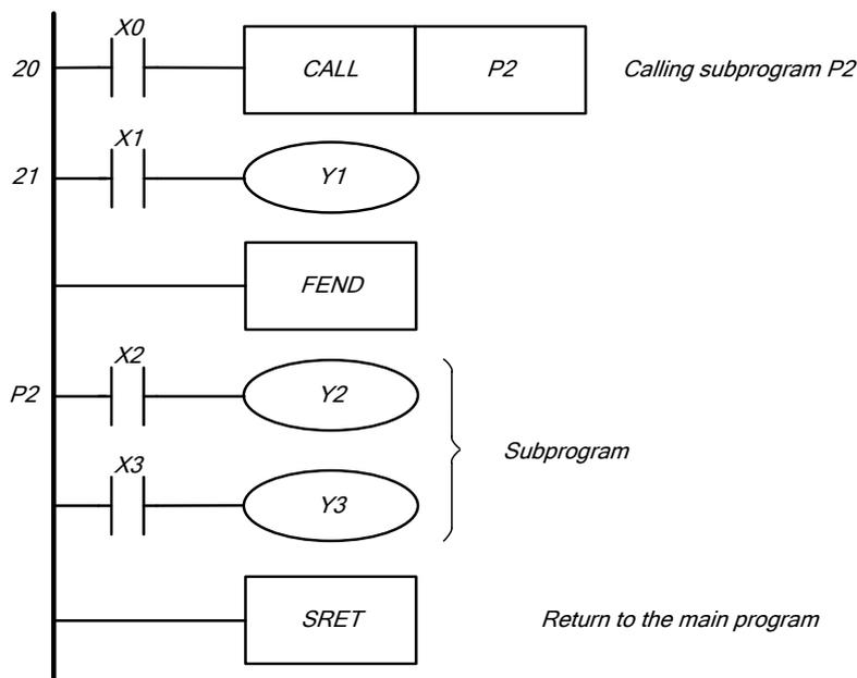
When  $X0 = 1$  at line 20 the program executing goes directly to the line marked P2, the subprogram executes, and after SRET command program executing returns to the line 21.
