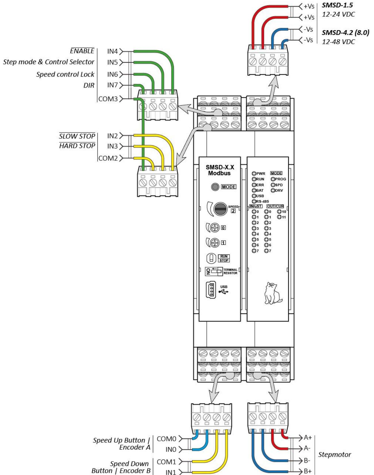
Fig. 3b – Terminal assignment – speed control mode
