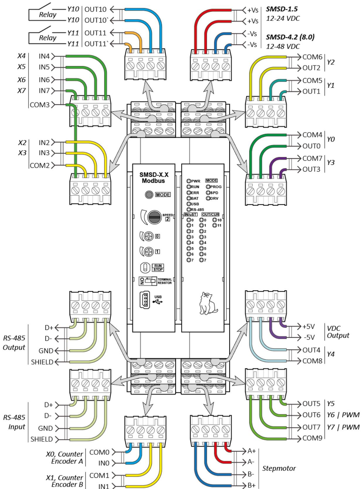
Fig. 4c – Terminal assignment – user program control mode
