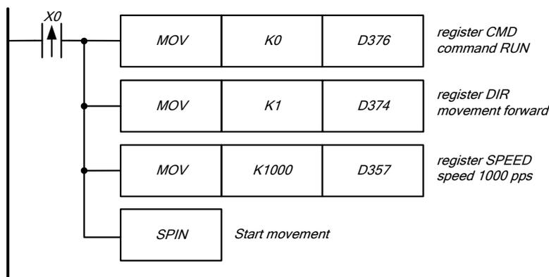
When the entry condition is satisfied, the motion command, direction and speed of rotation are set in the service registers. The followed instruction SPIN starts moving.
