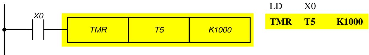
Upon condition  $X0 = 1$  the instruction TMR T5 counts until the value in the T5 register reaches the value of K1000 (100 sec). If  $X0 = 0$ , the execution of the TMR instruction will stop and T5 will reset to "0".
