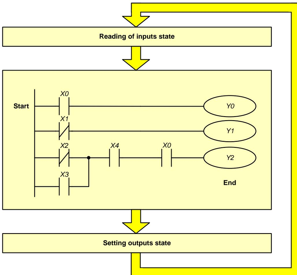
Fig. 13 – operation sequence in the controller
