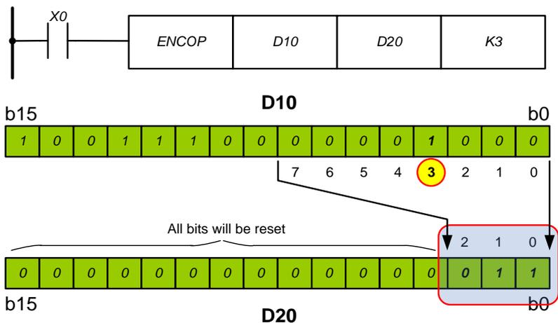
The 3d bit is on in the data register D10. So the value 3 is encoded and saved in the data register D20.
