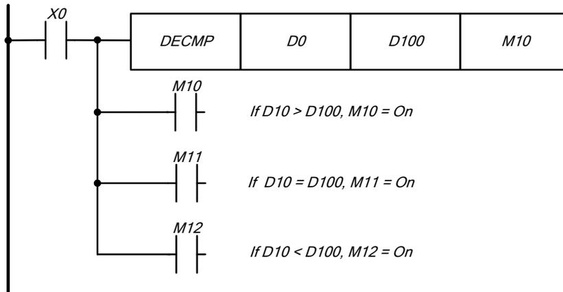
When contact X0 is turned on, the floating point number specified in D100 (S2) is compared with the floating point number specified in D0 (S1). If the number in D100 is less than the number D0, then the relay M10 is activated. If the number in D100 is equal to the number D0, then the relay M11 is turned on. If the number in D100 is greater than the number D0, then relay M12 is activated.
