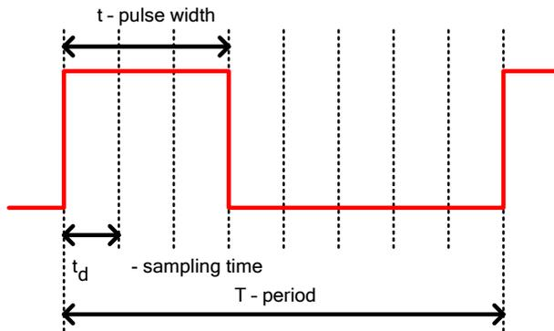
Let the sampling period be  $100 \mu\text{s}$ . When the input condition  $X0 = 1$  is satisfied, the PWM signal with a period of  $8 \times 100 \mu\text{s} = 0.8 \text{ ms}$  and a pulse duration of  $3 \times 100 \mu\text{s} = 0.3 \text{ ms}$  appears at the output Y6.
