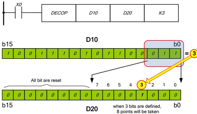
The lower 3 bits of the D10 data register are decoded. The decoding result  $1 + 2 = 3$  is transferred to the data register D20. The 3rd bit is turned on in this data register.
