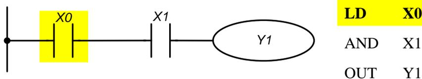
The instruction LD X0 "normally open contact X0" starts the sequential logic connection. If at the inputs X0 and X1 there is simultaneously a signal "1", then the output Y1 will be set to the state "1".
