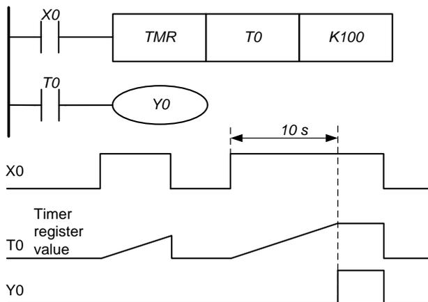
When the input X0 takes the state "1", the count of the set time begins. After reaching of the programmed 10 seconds, the output Y0 takes the state "1". The timer turns off and the T0 register is reset to zero as soon as the input X0 takes the state "0".
