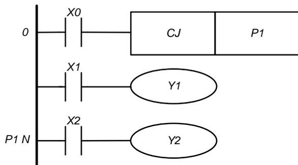
When  $X0 = 1$ , after the execution of line 0, the program immediately goes to the line with the pointer P1 and the lines located between them are not executed.
