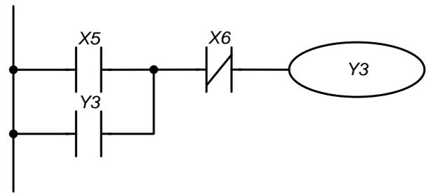
Fig. 12 – ladder diagram in the controller
