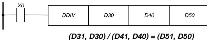
If X0 is turned on, division of data values in registers (D31, D30) and (D41, D40) is done. The result is saved in the data registers (D51, D50).
