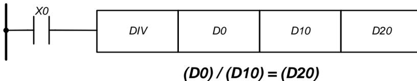
If X0 is turned on, division of data values in registers D0 and D10 is done. The result is saved in the data register D20.
