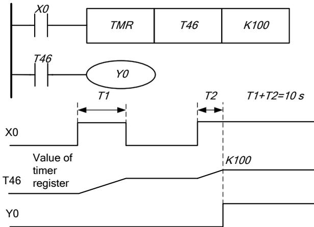
In addition to general purpose timers, the controller has accumulative timers, which, after disabling the control logical connection, save the accumulated time value.
