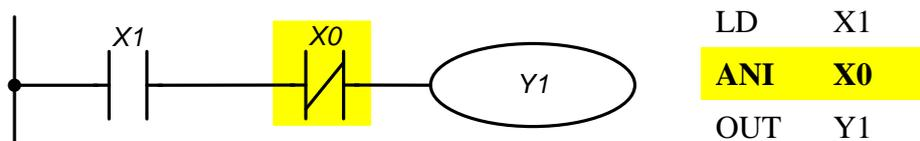
The instruction "Series connection - normally closed contact X0" creates a series logical connection with contact X1 and used to perform the logical operation NAND. If there is "1" at input X1 and "0" at X0, then output Y1 turns to the state "1".
