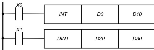
When input X0 is turned on, the floating point number in (D0, D1) is rounded to the nearest lower integer value. The result is saved in D10.
