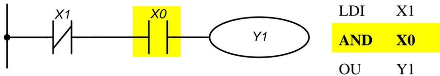
The instruction AND X0 "Series connection - normally open contact X0" creates a series logical connection with contact X1 and used to perform the logical multiplication operation. If there is "0" at input X1 and "1" at X0, then output Y1 turns to the state "1".
