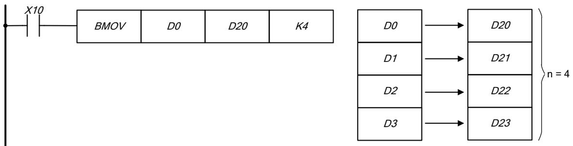
If X10 is turned on, the values of registers D0 – D3 is transferred to the registers D20 – D23.
