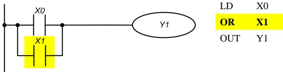
The instruction "Parallel connection – normally open contact X1" creates a parallel logical connection with contact X0 and used to perform the operation of logical addition. If at least one of the inputs X0 or X1 is "1", then the output Y1 turns to the state "1".
