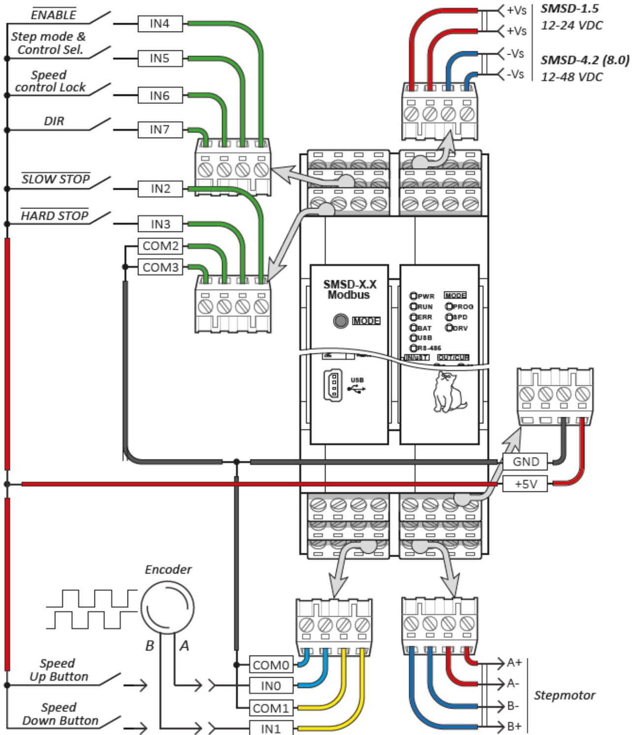
Fig. 35 – Connection of control elements
