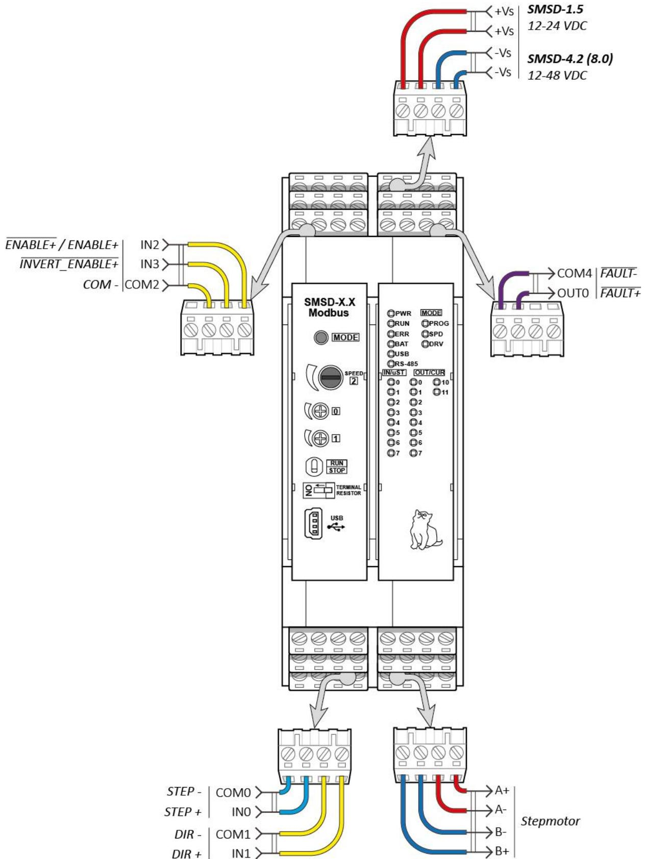
Fig. 2a – Terminal assignment – driver control mode
