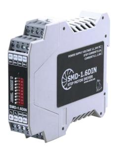
SMD-1.6DIN is a driver for small and medium size stepper motors. The driver provides smooth operation and good speed-torque performance. The driver has the STO (Safe Torque Off) function which provides motor phases deenergizing in case of any alarm situation.
