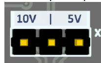
Fig.14. – a jumper for selecting the analog signal range.
