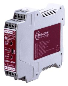
SMD 4.2DIN ver.3 is a stepper motor driver designed to control two and four-phase hybrid stepper motors. The controller provides an excellent motor dynamics and high torque performance. This model provides 2 control methods: STEP/DIR positioning and analog speed control.
