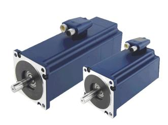
High-torque stepper motor with M12 connector with protection class IP65 (except shaft output) in size NEMA 34 (86 mm) and 1.8° step angle (full step). Identical flange size as the standard motor ST8918, therefore electrically and mechanically interchangeable.
