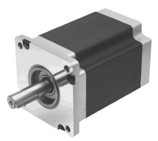
High-torque stepper motor in size NEMA 42 (110 mm) with 1.8° step angle (full step). Ideal solution for direct drives because of its high torque in relation to the motor size.
