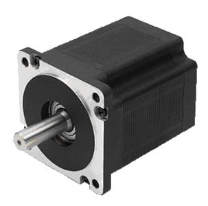
High-torque stepper motor in size NEMA 34 (86 mm) with 1.8° step angle (full step). Ideal solution for direct drives because of its high torque in relation to the motor size.
