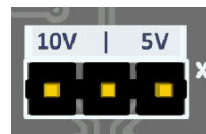
Fig.14. – jumper for selecting the analog signal range.
