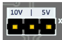
Fig.14. – jumper for selecting the analog signal range.
