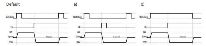
Operation logic of the inputs "START/STOP" and "DIR" can be adjusted with the jumpers "START\_PIN" and "DIR\_PIN" – fig. 5.
