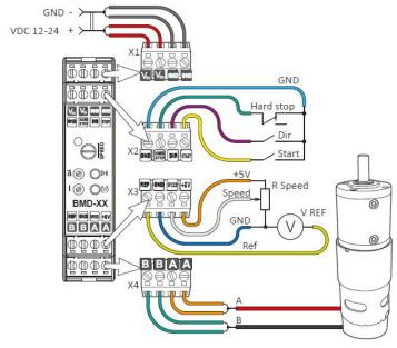
Fig.2. BMD-20DIN connection scheme (example of speed control by an external potentiometer.)
