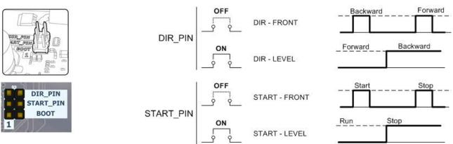
Fig. 5. START\_PIN and DIR\_PIN jumpers
