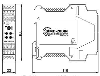
Fig.1 Dimensions of BMD-20DIN
