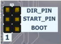
Fig. 5. START_PIN and DIR_PIN jumpers
